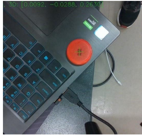
Fig. 6. Computer vision tracking the red target and calculating the 3D position
